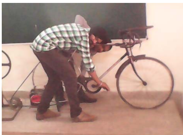
Fig. 2: Handle power system for battery charging.
